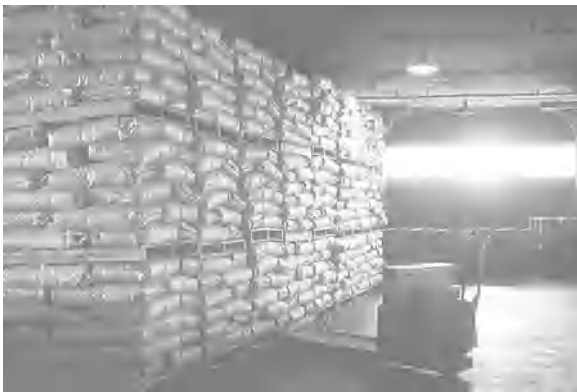
The design of the floor system of this warehouse building must account for critical locations of storage materials on the floor. Influence lines must be used for this purpose. (Photo courtesy of Portland Cement Association.)
