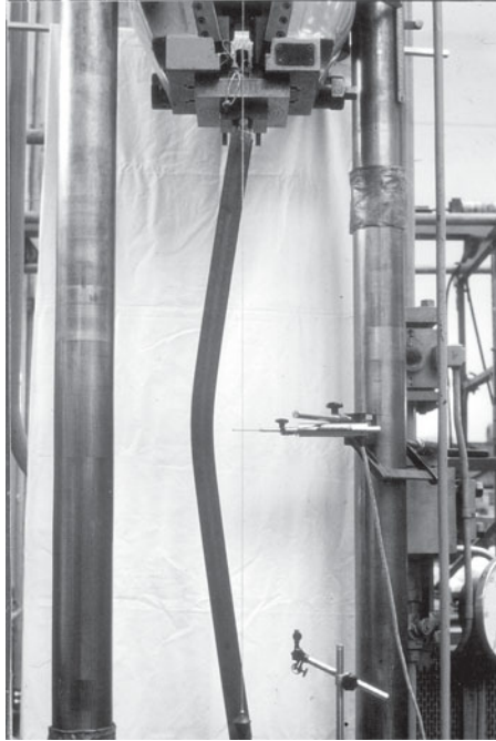
Buckling of a pin-ended column in a laboratory test (Courtesy: Late Dr. W. Kurth of Germany)
