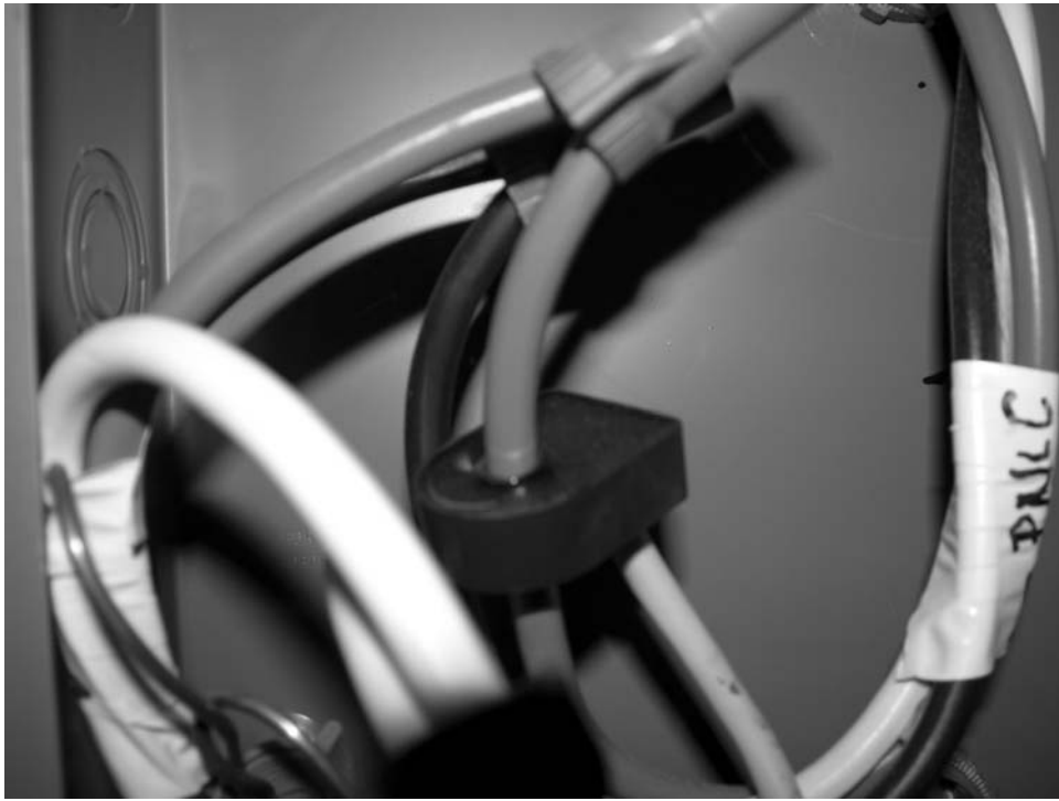
Figure 13.5 The current Toroid sensor.
