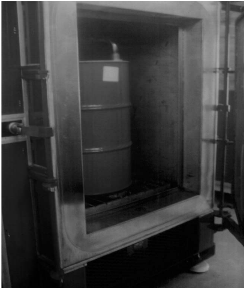
Figure 14.3 Residential prototype steam reforming of waste.
