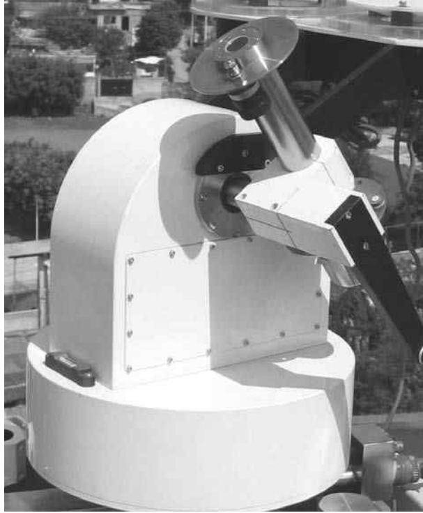
FIGURE 2.26 Pyrheliometer. (Courtesy of CIE-UNAM.)
