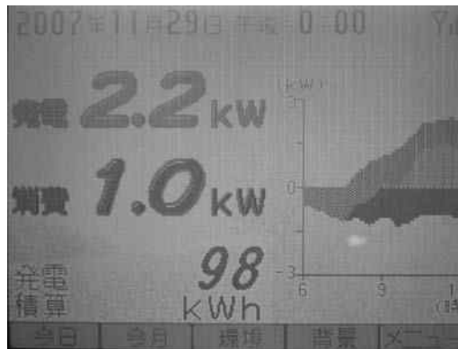
FIGURE 8.7 Consumer-friendly Kyocera residential PV meter display
