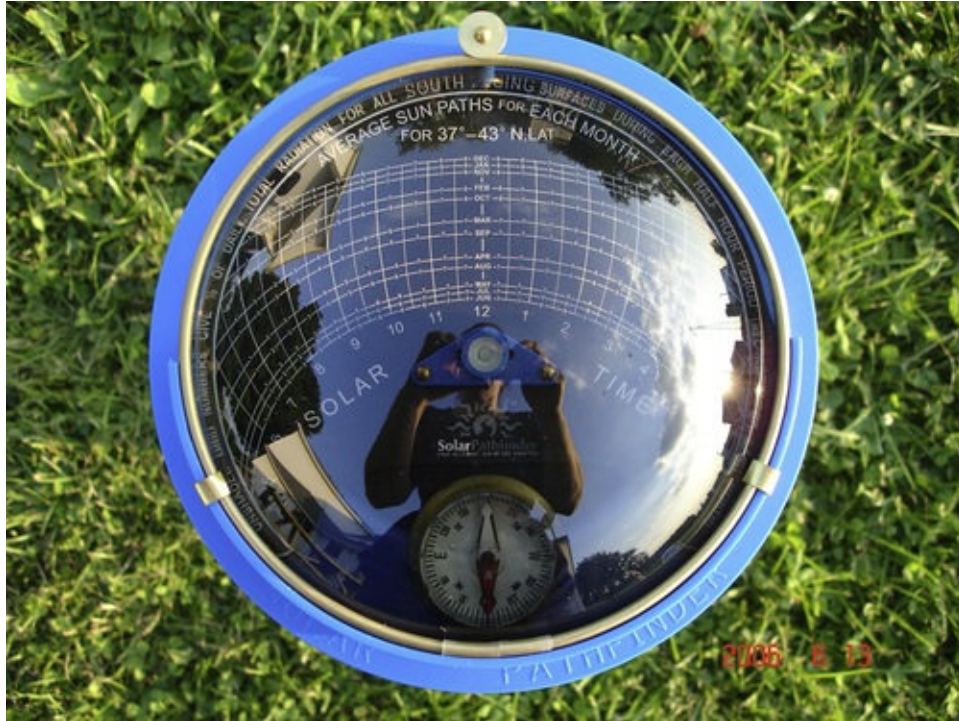
FIGURE 2.15 Solar Pathfinder. Photo courtesy of The Solar Pathfinder Company. (For color version of this figure, the reader is referred to the online version of this book.)
