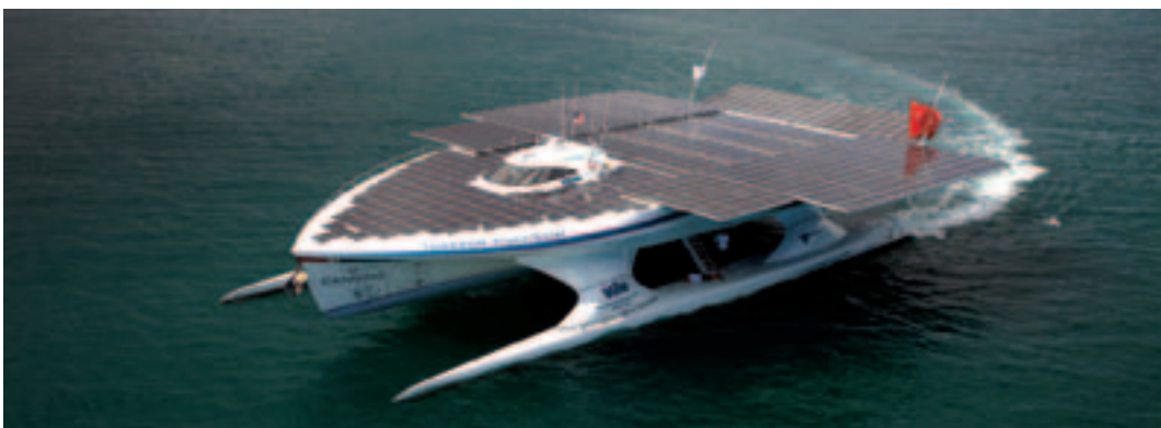
Photo 5.4 This 31-m demonstration boat is circumnavigating the globe, powered only by its PV panels
