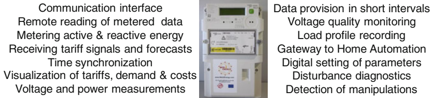
Fig. 6.33 Smart metering functions
