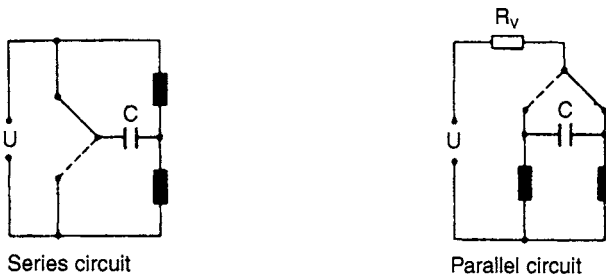
Figure 5.10 Circuit for the generation of the phase-shifted voltages for the synchronous motor of Figure 5.9
