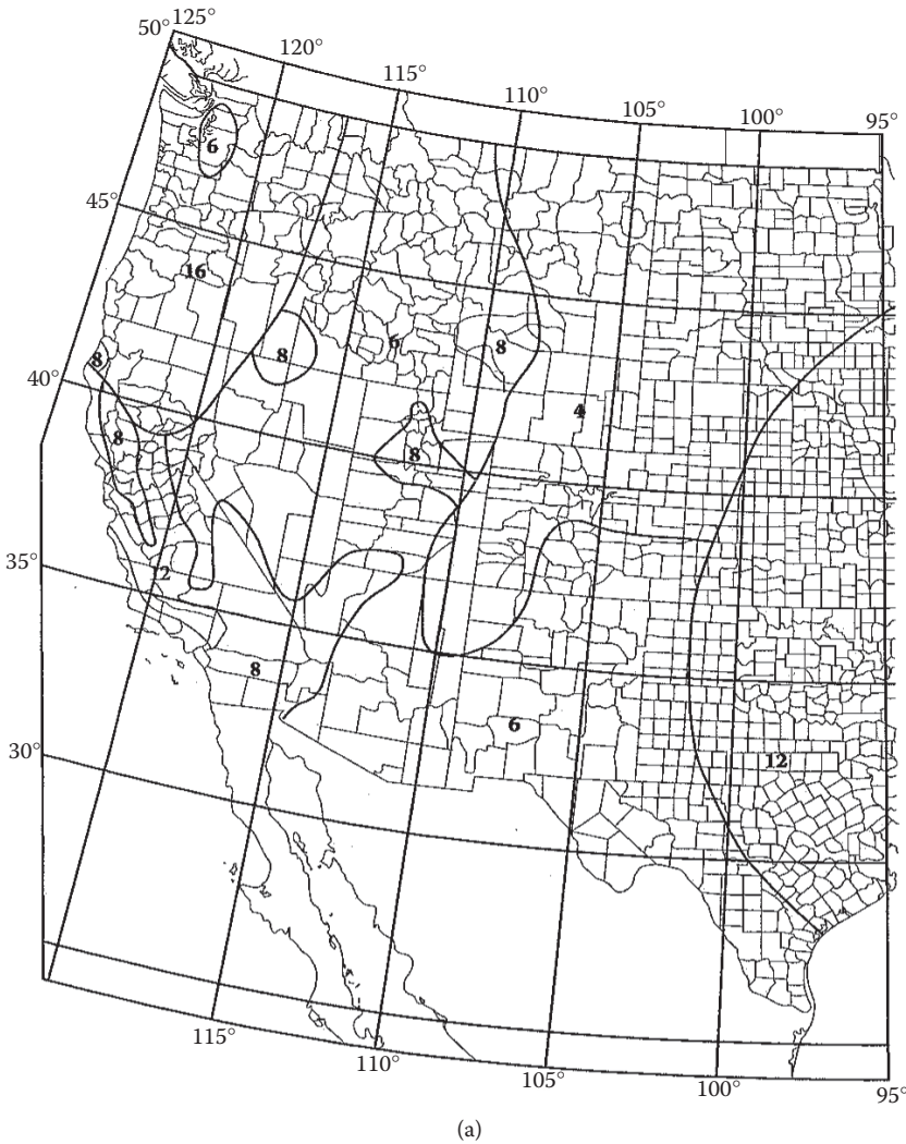
FIGURE 5.5 Long-period transition period, T_L . (a) and (b) divide the country in two halves. (Courtesy of American Society of Civil Engineers, Reston, VA.)
