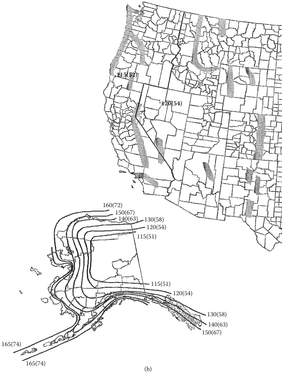
FIGURE 4.3 (Continued) Basic wind speed for risk category III and IV buildings. (a) and (b) simply divides the country in two halves. Notes: 1. Values are nominal design 3-second gust wind speeds in miles per hour (m/s) at 33 ft. (10 m) above ground for exposure C category. 2. Linear interpolation between contours is permitted. 3. Islands and coastal areas outside the last contour shall use the last wind speed contour of the coastal area. 4. Mountainous terrain, gorges, ocean promontories, and special wind regions shall be examined for unusual wind conditions. 5. Wind speeds correspond to approximately a 3% probability of exceedance in 50 years (Annual Exceedance Probability = 0.000588, MRI = 1700 years). (Courtesy of American Society of Civil Engineers.)
