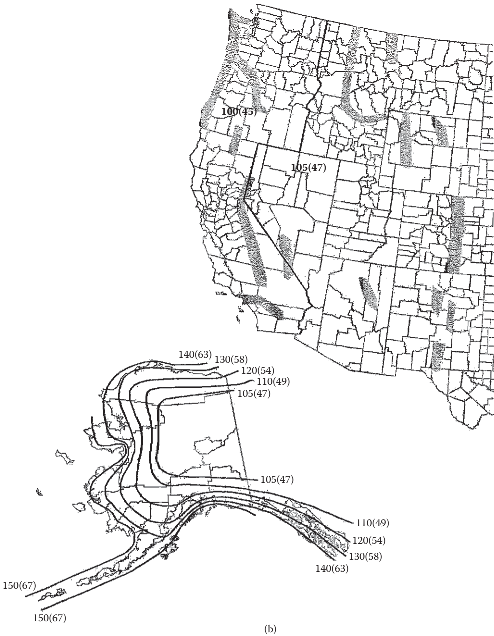
FIGURE 4.1 (Continued) Basic wind speed for risk category I buildings. (a) and (b) simply divides the country in two halves. Notes: 1. Values are nominal design 3-second gust wind speeds in miles per hour (m/s) at 33 ft. (10 m) above ground for exposure C category. 2. Linear interpolation between contours is permitted. 3. Islands and coastal areas outside the last contour shall use the last wind speed contour of the coastal area. 4. Mountainous terrain, gorges, ocean promontories, and special wind regions shall be examined for unusual wind conditions. 5. Wind speeds correspond to approximately a 15% probability of exceedance in 50 years (Annual Exceedance Probability = 0.00333, MRI = 300 years). (Courtesy of American Society of Civil Engineers.)
