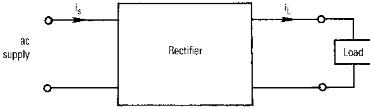
FIG. 1 General rectifier representation.
