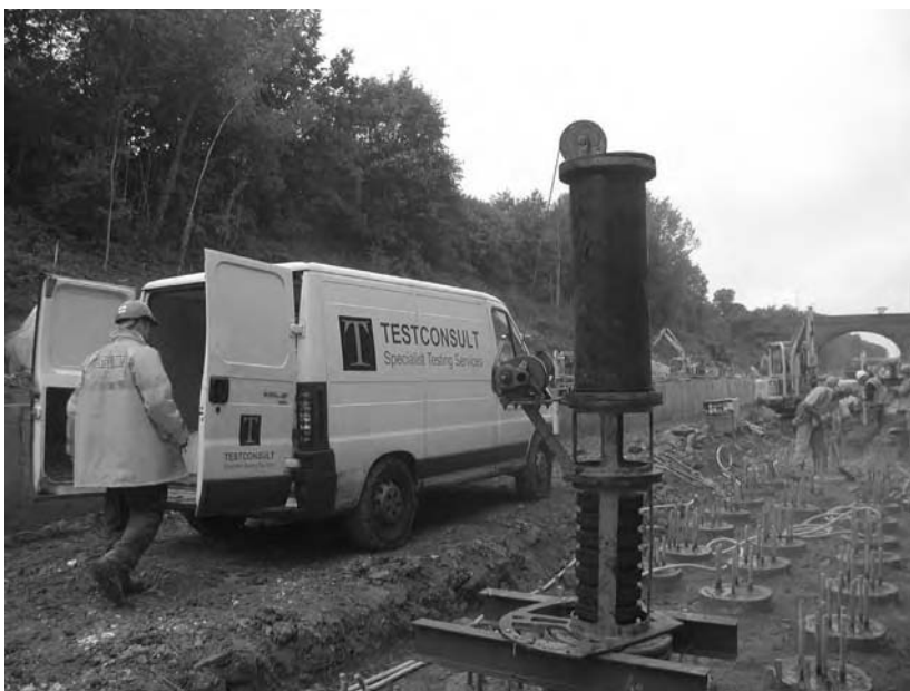
Figure 11.21 SIMBAT test using a mini rig for small diameter dynamic tests (courtesy Test Consult).
