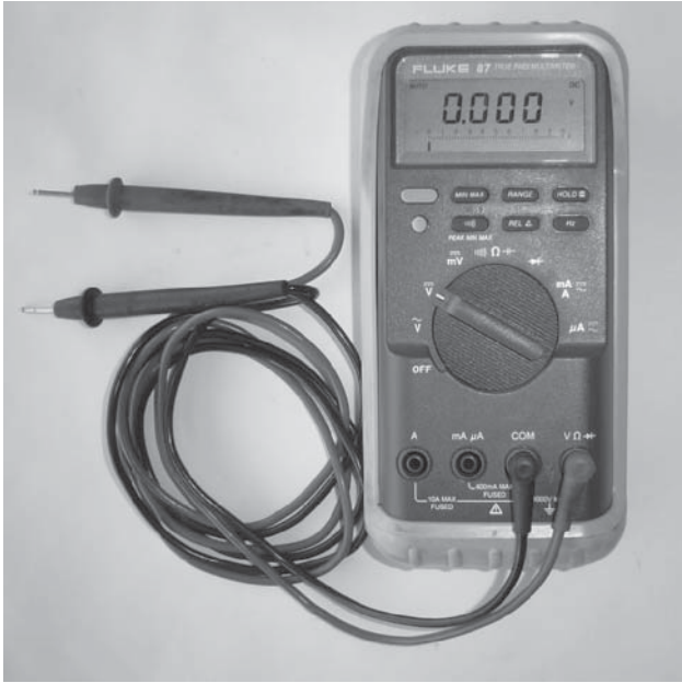
Figure 2-23 Digital multimeter with test leads attached for a voltage measurement.
