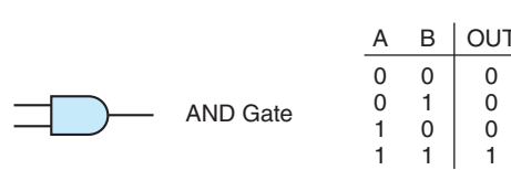
Figure 11-34 AND gate symbol and truth table.
