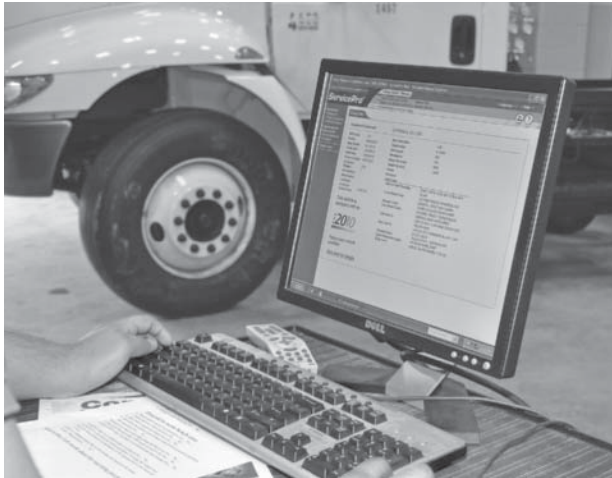
Figure 12-31 Electronic service tool used to modify ECM programmable parameters after tire size or rear-axle ratio change.
