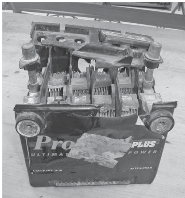
Figure 1-6 Lead-acid battery after a spark caused an explosion.
