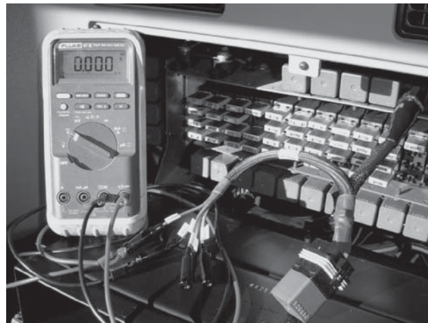
Figure 4-37 Relay breakout T used to test ISO relays and relay circuits.
