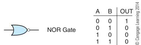
Figure 11-39 NOR gate and truth table.
