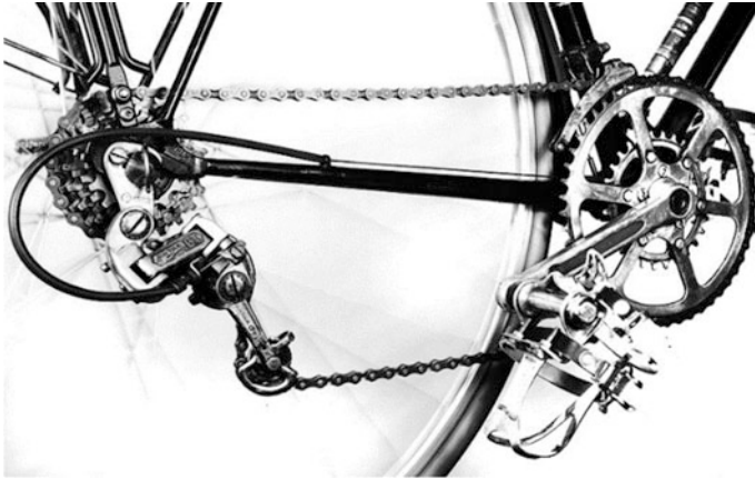
Fig. 4 Derailleur mechanism for changing sprockets sizes, Brown [33]
