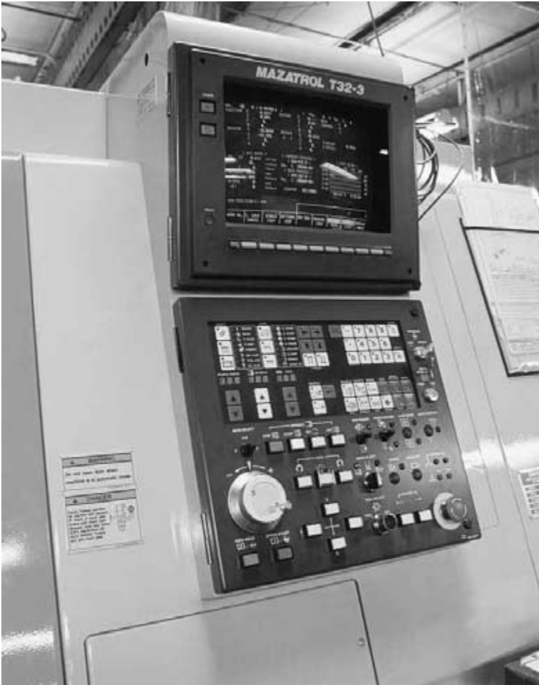
FIGURE 5.2b Turning center control panel.
