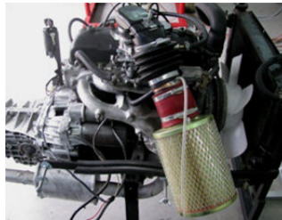
Figure 47. Super absorbing cylindrical filter with internal diffuser trial
