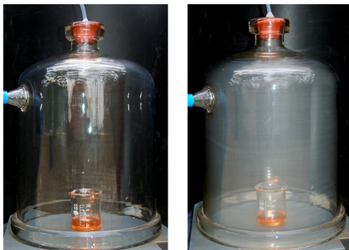
Figure 2. A picture of the bell jar with discharge (left) and without discharge (right).
