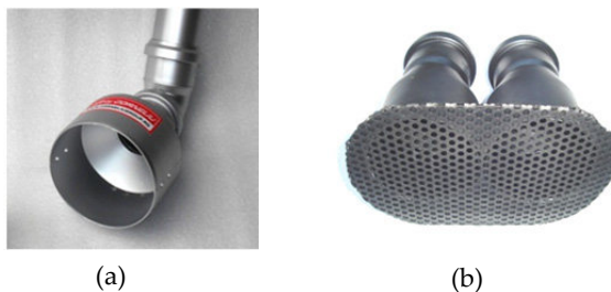
Figure 21. External collector diffusers - physical models
