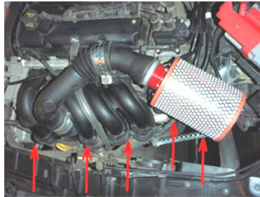
Figure 36. Filter assembly without the cooling radiator's integrated deflector
