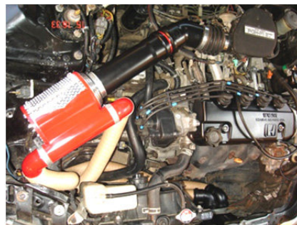
Figure 27. DATD, bi-route mounted on Honda Civic, 1.6
