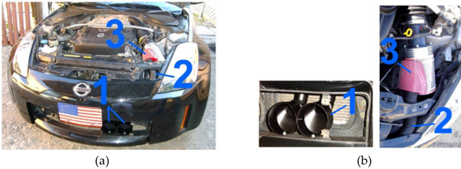
Figure 24. a - DATD mounted on the engine; b - component parts: 1 - external collector diffusers, 2 - pipe connection, 3 - bi-route axial external collector
