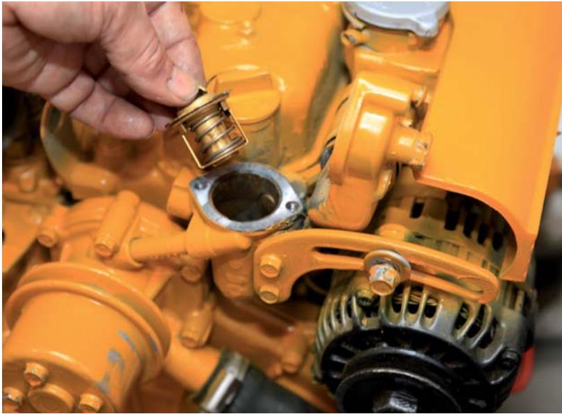
Removing a thermostat.
