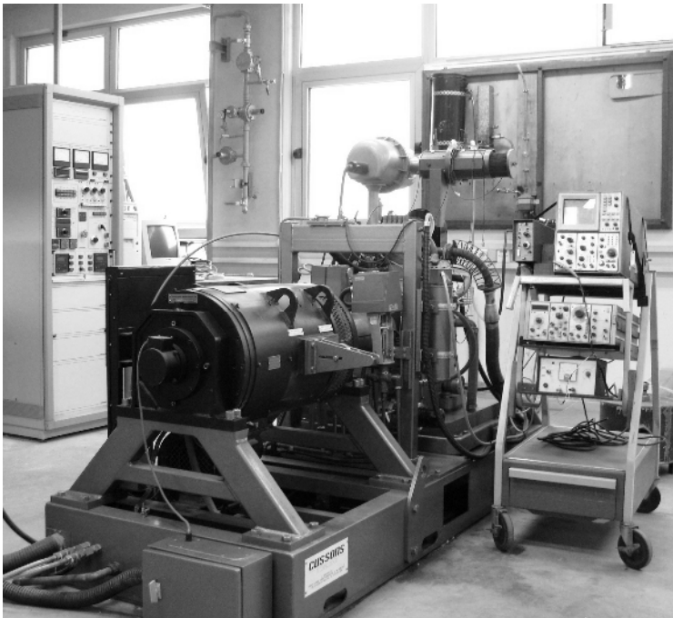
Figure 4.2. Photograph of a transient engine test bed
