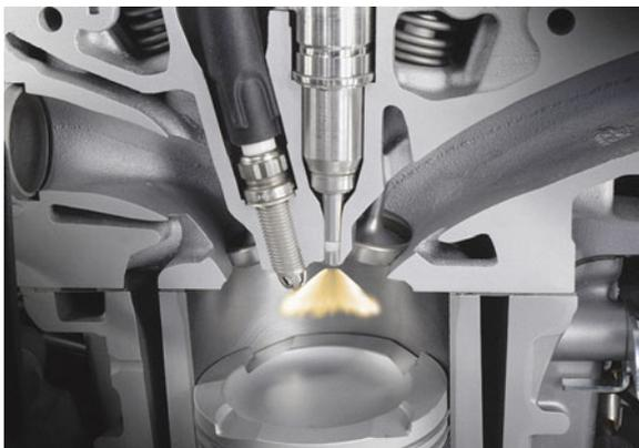
advantage of efficiency. Typical values of  $\epsilon$  for current direct-injecting naturally aspirated engines are around 12, and 10–10.5 for turbo engines.
