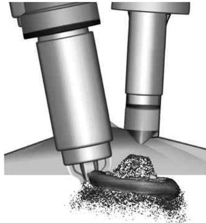
mixture directly at the edge of the spray at the spark plug position is thus a top prerequisite of a reliable ignition. Then, the detour via the piston recess is superfluous, as is most of the efficiency-lowering fuel wetting of the piston. HC emissions can be significantly reduced to the level of good stoichiometrically operated engine (Fig. 4.39).
