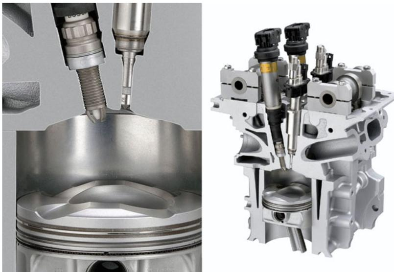
**Fig. 4.36** Example of the central injector arrangement of a spray guided combustion process, BMW Presseinformation
