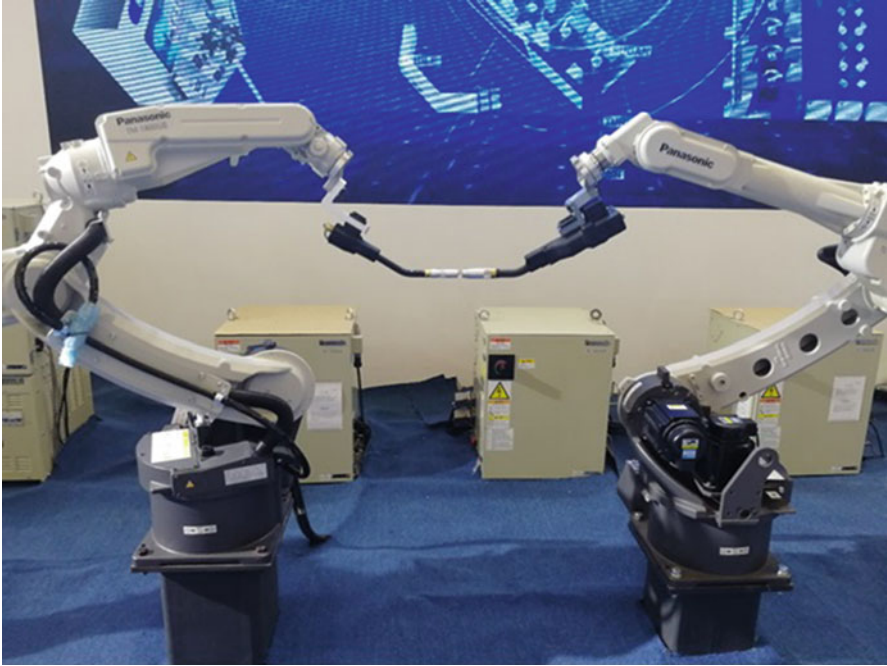
Fig. 4.7 Cooperative welding robot
